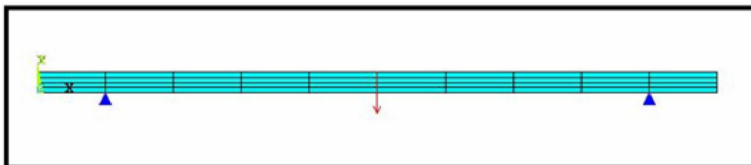
Figure 4 Mesh Generation of the Composite Beam.
