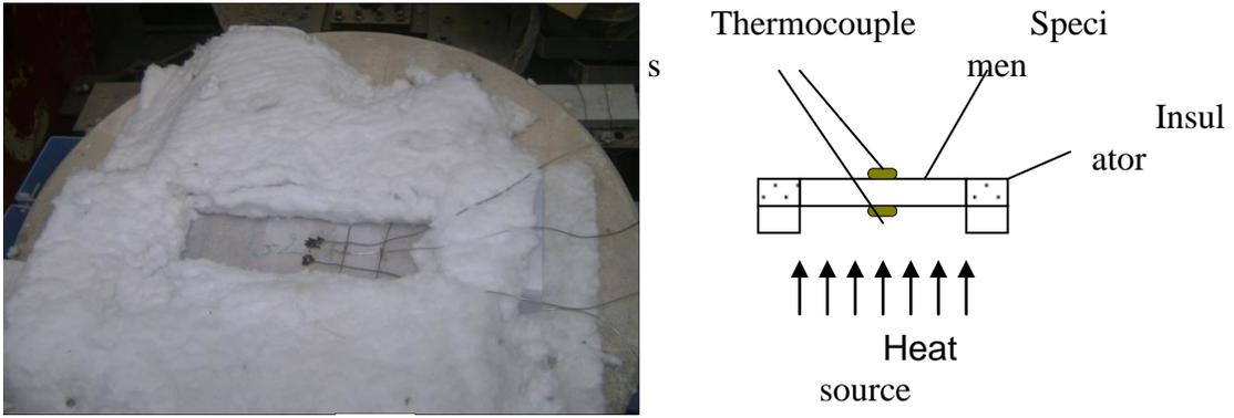
Figure 1 Heat transfer test
