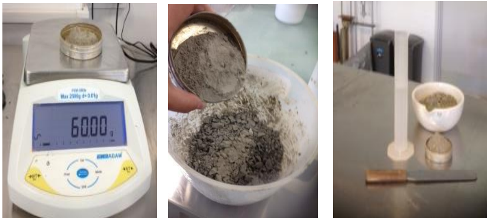
Figure (3): Mixing soil with cement
