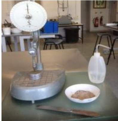
Figure (4): Penetrometer and equipment for liquid limit experiment.
