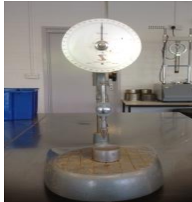
Figure (4): Penetrometer and equipment for liquid limit experiment.
