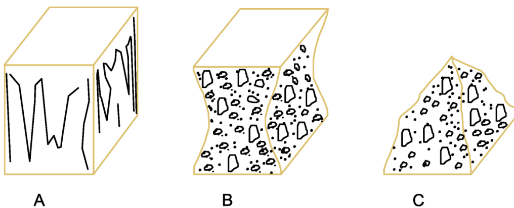
Figure (4): Satisfactory compression failure modes [35]: A- Cracks failure, B- Damage failure and C-Explosive failure
