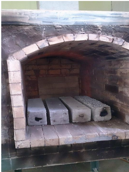
Figure (3): Gradually Cooling of Specimens.
