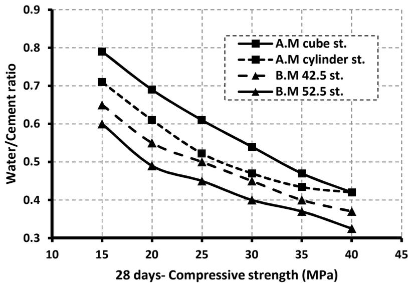
**Figure 5: Compressive strength-W/C ratio relationship for concrete mixes using uncrushed aggregate.**
