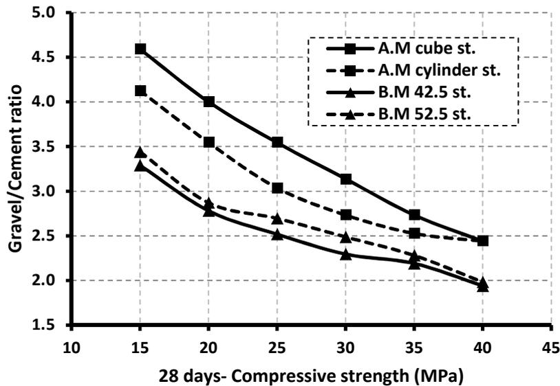
**Figure 8: Compressive strength-Gravel/Cement ratio relationship for concrete mixes using crushed aggregate.**
