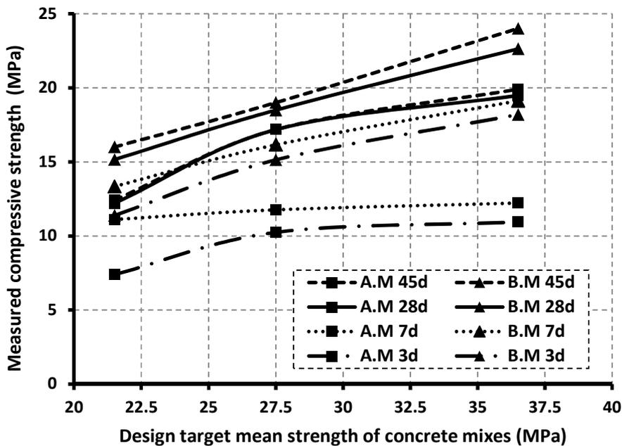
Figure 15. Values of compressive strength for various concrete mixes containing uncrushed aggregate
