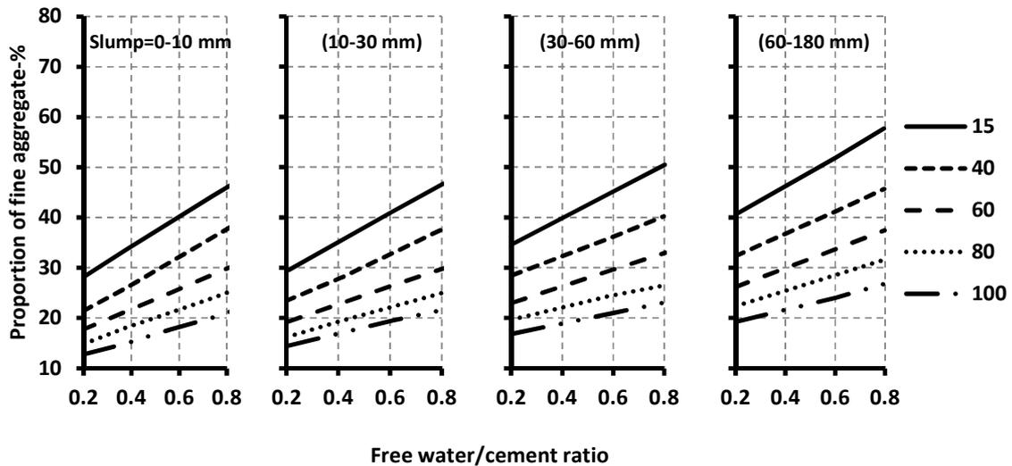
Figure 3: Recommended proportions of fine aggregate according to percentage passing a 600 µm sieve [10].
