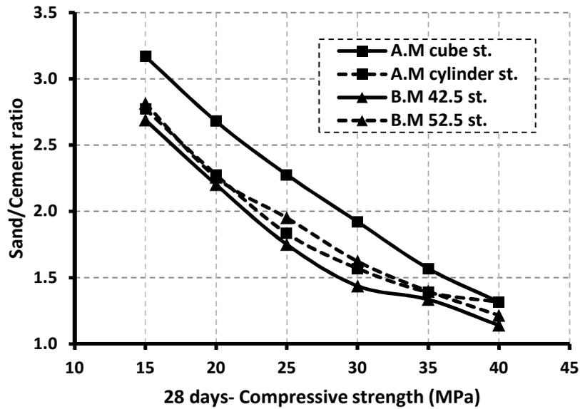
Figure 6: Compressive strength-Sand/Cement ratio relationship for concrete mixes using crushed aggregate.
