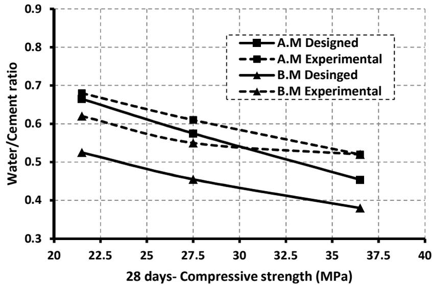
Figure 12. Water/ Cement ratio for various concrete mixes containing uncrushed aggregate
