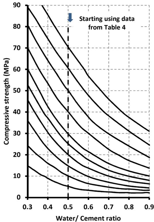
**Figure 1: Relationship between compressive strength and free-water/cement ratio [10].**
