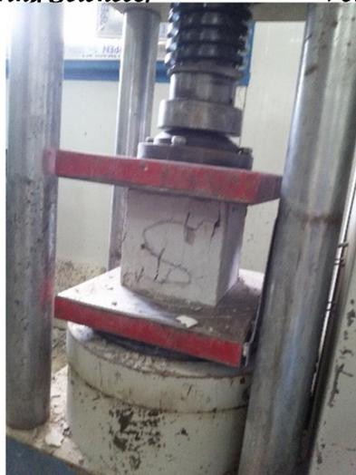
**Figure 11. Digital controlled compression machine used in compressive strength test**
