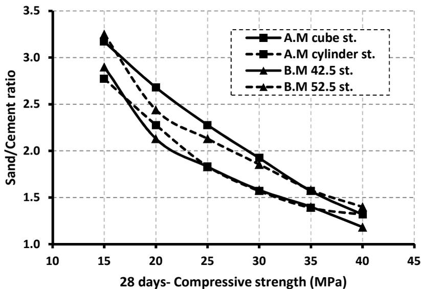
Figure 7: Compressive strength-Sand/Cement ratio relationship for concrete mixes using uncrushed aggregate.
