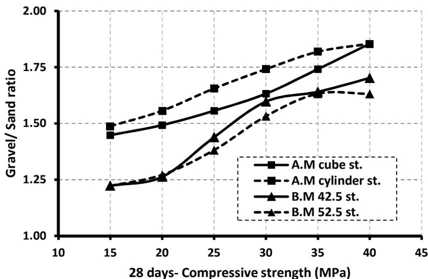
**Figure 16. Compressive strength-Gravel/sand ratio relationship for concrete mixes using crushed aggregate.**
