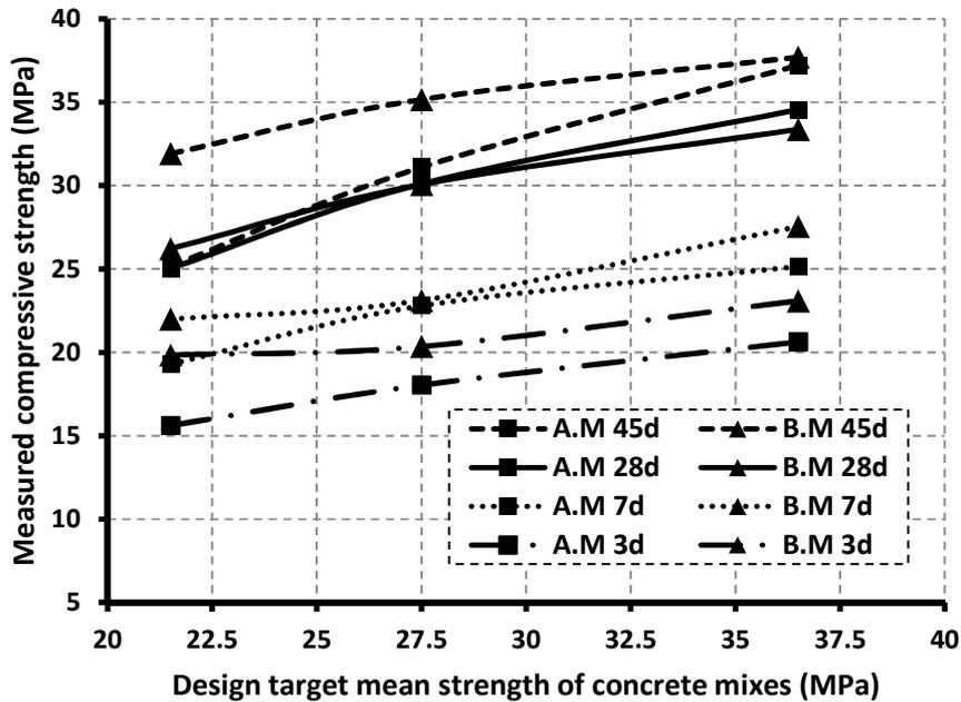
Figure 14. Values of compressive strength for various concrete mixes containing crushed aggregate
