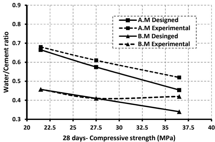
Figure 13. Water/ Cement ratio for various concrete mixes containing uncrushed aggregate
