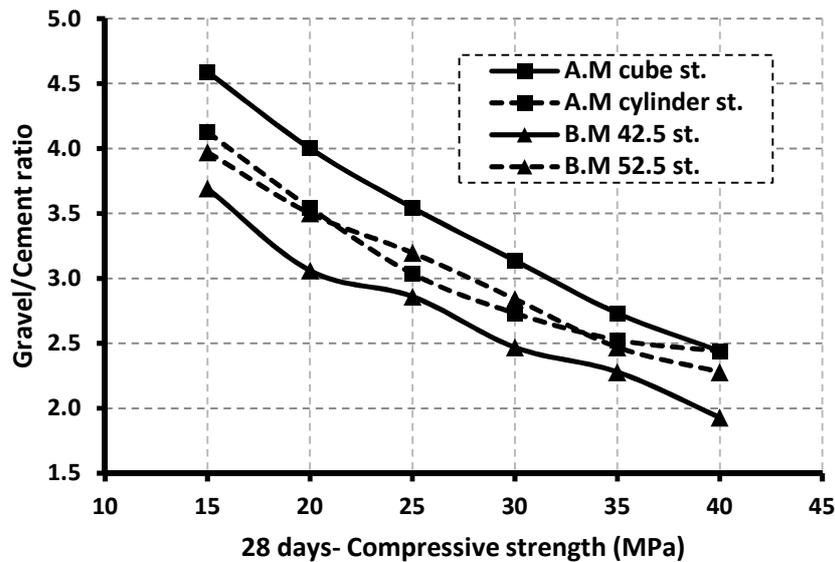
**Figure 9: Compressive strength-Gravel/Cement ratio relationship for concrete mixes using uncrushed aggregate.**
