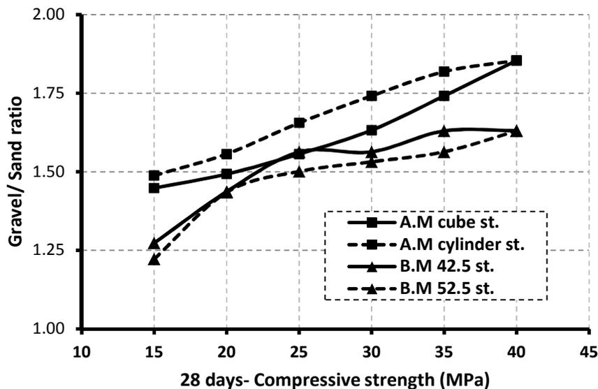
Figure 17. Compressive strength-Gravel/sand ratio relationship for concrete mixes using uncrushed aggregate.
