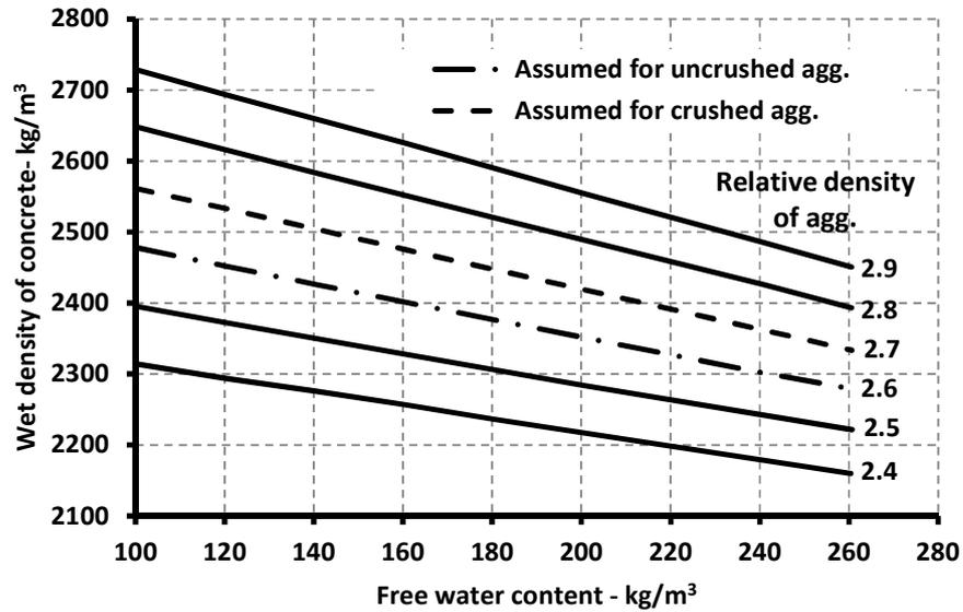
Figure 2: Estimated wet density of fully compacted concrete [10].
