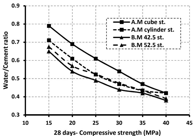
**Figure 4: Compressive strength-W/C ratio relationship for concrete mixes using crushed aggregate.**
