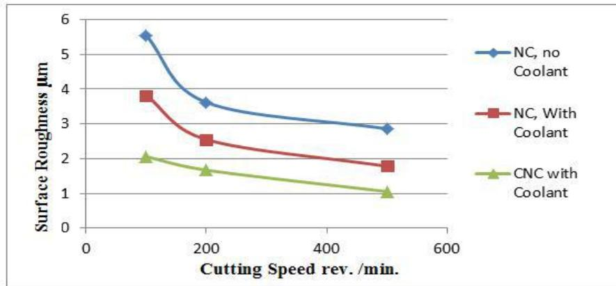
Figure (5) Relation between cutting speed and surface roughness, Depth of cut was fixed on 1 mm feed on 0.064 mm/rev.
