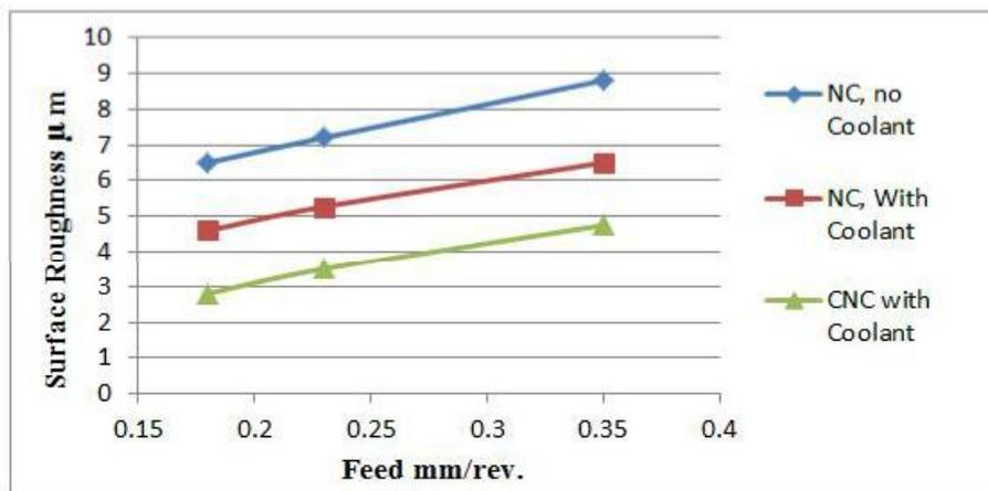
Figure (7) Relation between feed and surface roughness, cutting speed was fixed on 250 rev./min. and depth of cut 1 mm
