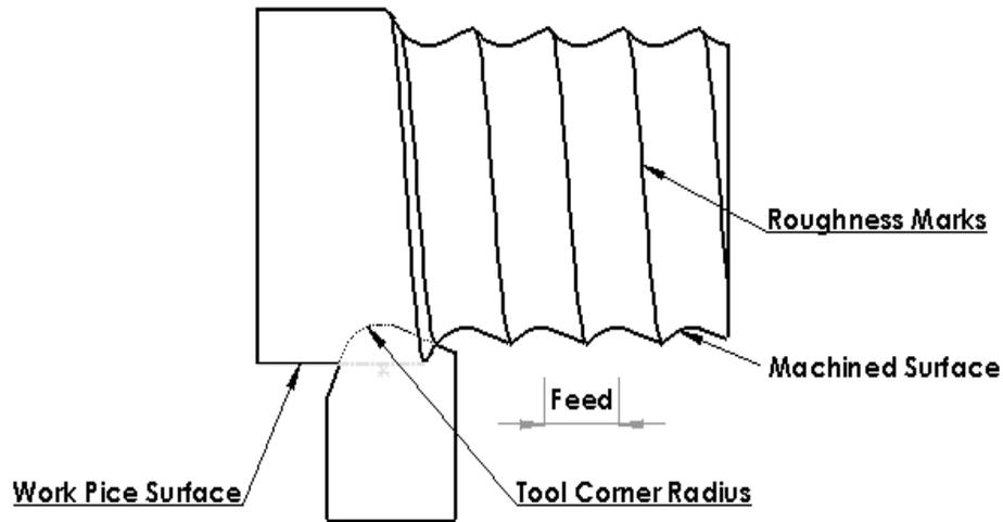
Figure (1) Ideal surface roughness due to tool feed
