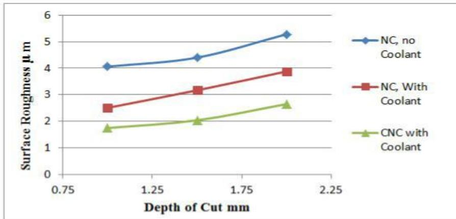
Figure (6) Relation between depth of cut and surface roughness, cutting speed was fixed on 160 rev./min. and feed 0.05 mm/rev.
