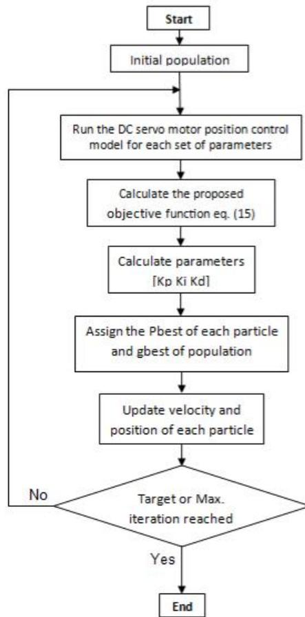
Figure (3): PSO-PID algorithm flowchart
