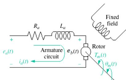
**Figure (1):** Equivalent circuit of armature control of DC servomotor
