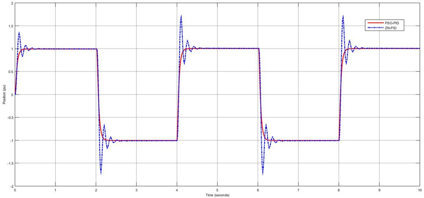
Figure (7): DC servomotor response to step change of input reference
