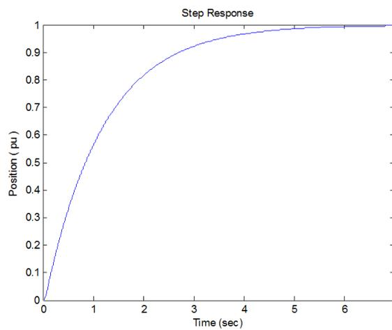
Figure (4): DC servo motor step response
