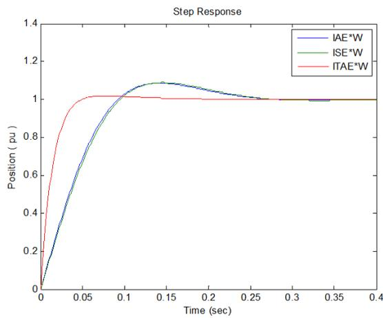
Figure (6): Position step response of DC motor using proposed objective function
