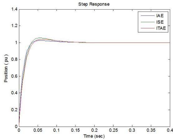
Figure (5): position step response of DC servo motor using common performance criteria
