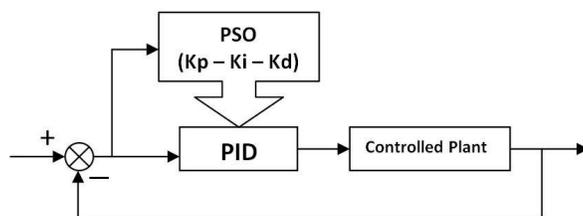
**Figure (2):** PSO-PID controller
