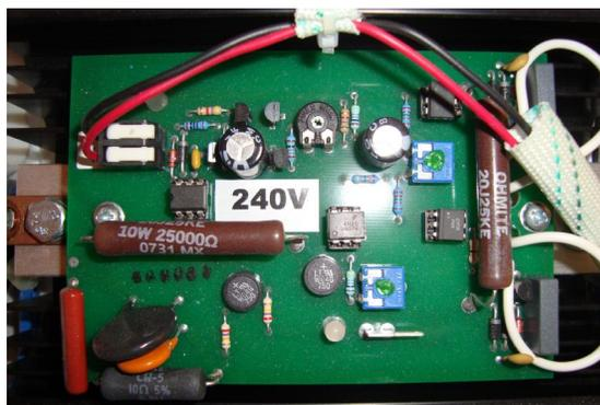
Fig. 11: A real photo for the SCR power controller (actuator)
