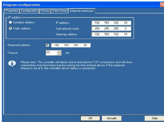
Fig.9 IP setting of Ethernet module
