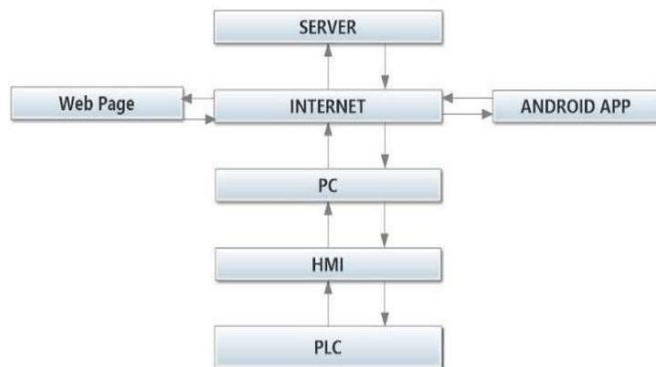
Figure 2: Connection diagram of the PLC to the Internet
