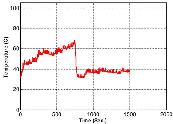
Fig.14: The real-time response of the PID temperature control system for two set points: 65°C and 40°C
