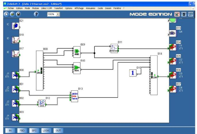
Fig. 10: The four I/O words accessible by the Ethernet communication module
