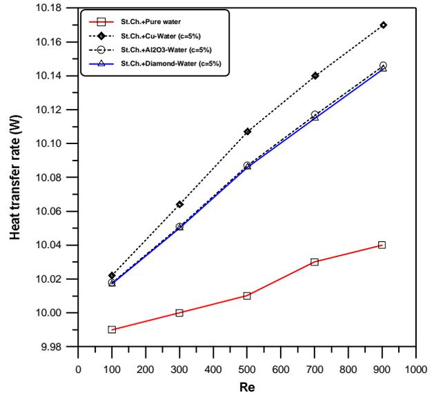
Fig. 17 variation of total heat transfer rate with Re for straight channels with pure water and three types of nanofluids
