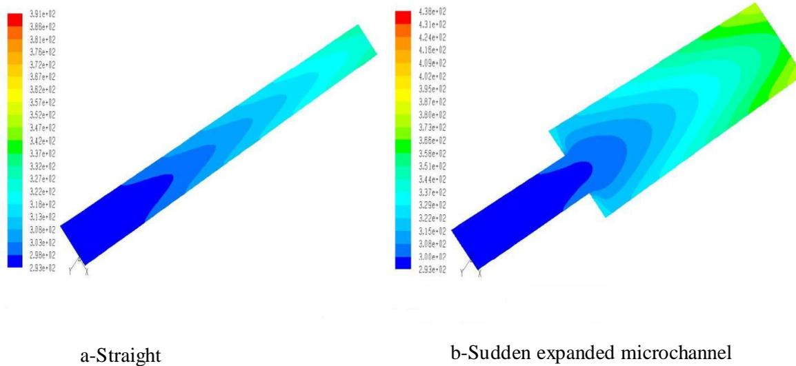
Fig. 5 Temperature contour at longitudinal central plan ( $y=0.00005m$ ),  $Re=100$
