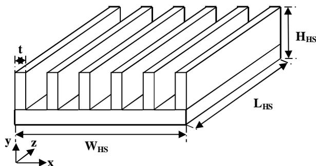
Fig. 1 schematic of microchannel heat sink with straight rectangular microchannels
