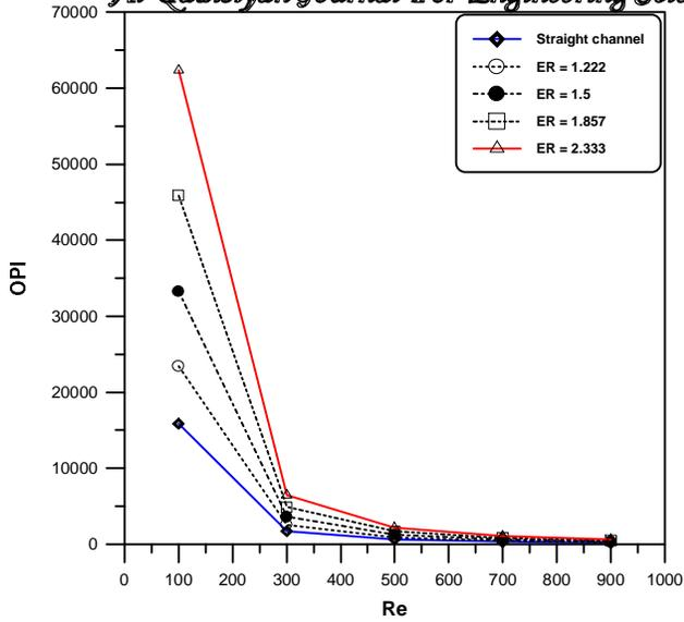
Fig. 8 variation of overall performance index with Re for straight and expanded channels
