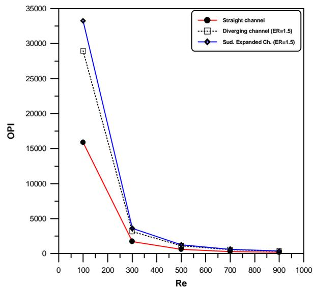
Fig. 13 variation of OPI with Re for straight, diverged and sudden expanded channels
