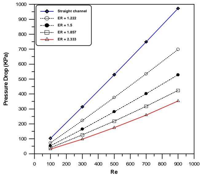
Fig. 7 variation of total pressure drop with  $Re$  for straight and sudden
