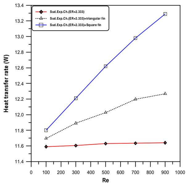
Fig. 14 variation of total heat transfer rate with Re for sudden expanded channels with triangular and square fins
