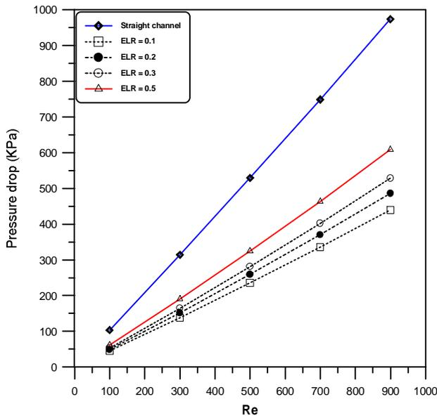
Fig. 10 variation of total pressure drop with Re for straight and sudden expanded channels with different expansion length ratio
