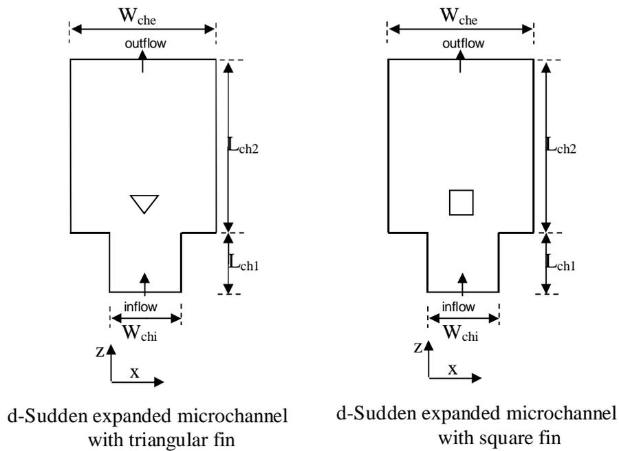
Fig.2 schematics of studied channels configurations (top view)
