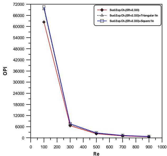
Fig. 15 variation of OPI with Re for sudden expanded channels with triangular and square fins
