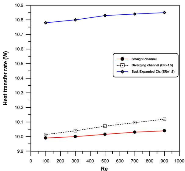
Fig. 12 variation of total heat transfer rate with Re for straight, diverged and sudden expanded channels
