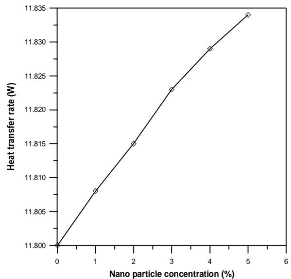
Fig. 19 variation of total heat transfer rate with c for sudden expanded channel with square fin and Cu-water nanofluid
