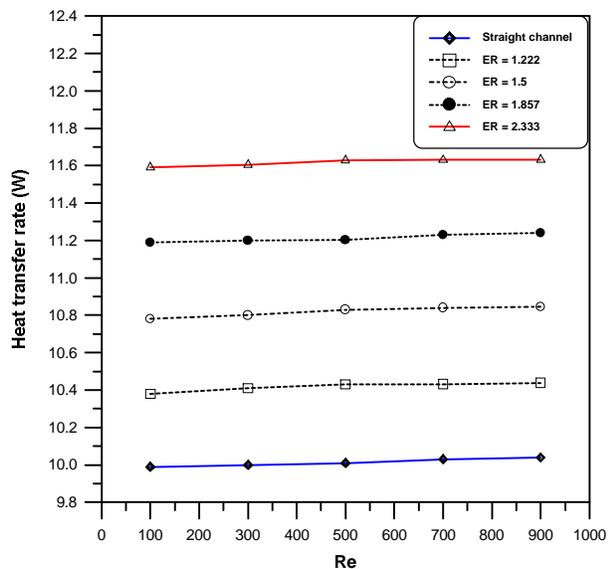
Fig. 6 variation of total heat transfer rate with  $Re$  for straight and sudden expanded channels
