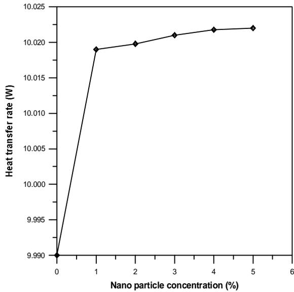
Fig. 16 variation of total heat transfer rate with c for straight channel with Cu-water nanofluid
