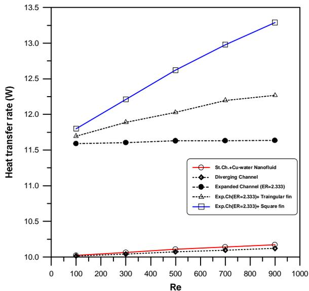
Fig. 18 variation of total heat transfer rate with Re for different cases studied
