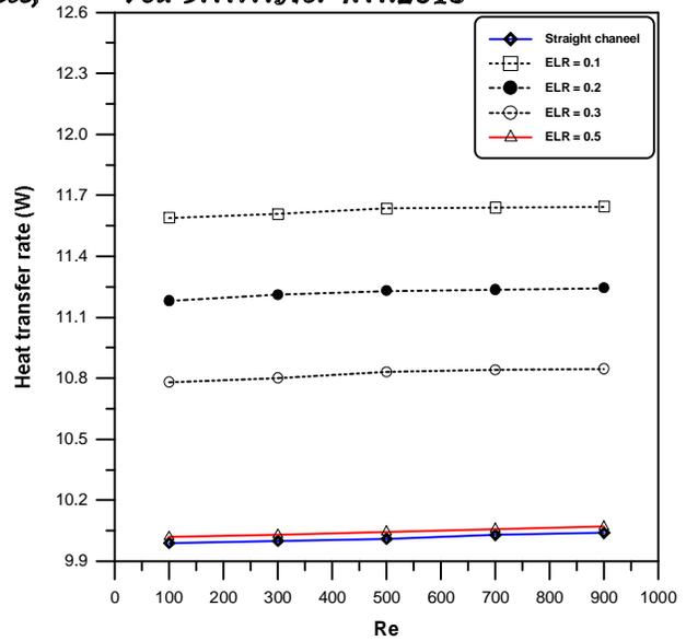
Fig. 9 variation of total heat transfer rate with Re for straight and sudden expanded channels with different expansion length ratio
