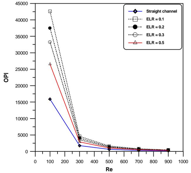
Fig. 11 variation of overall performance index with Re for straight and sudden expanded channels with different expansion length ratio
