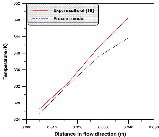
Fig. 3 variation of wall temperature in flow direction as a comparison between present model and [18]
