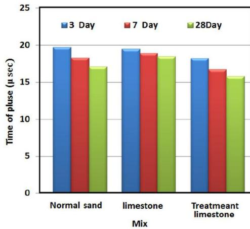
Figure (8): The relationship between mix and ultrasonic pulse velocity.
