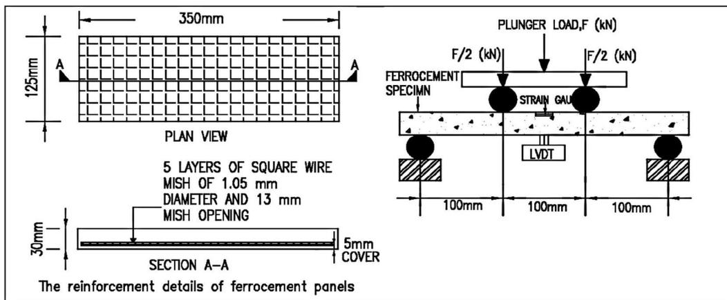
**Figure (2):** Details of ferrocement panels and test.
