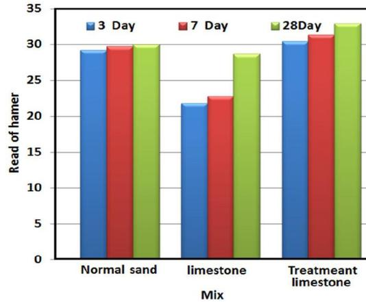
Figure (9): The relationship between mix and read of hammer.
