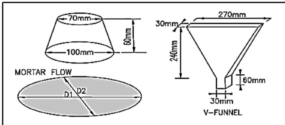
Figure (3): Dimensions of mini-slump and mini V-funnel.
