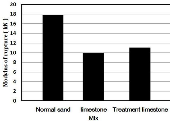
Figure (10): The relationship between mix and modulus of rupture for prism.
