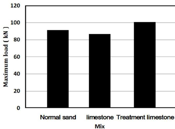
Figure (12): The relationship between mix and maximum load.
