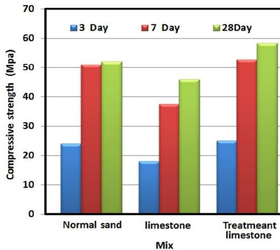
Figure (7): The relationship between mix and compressive strength.
