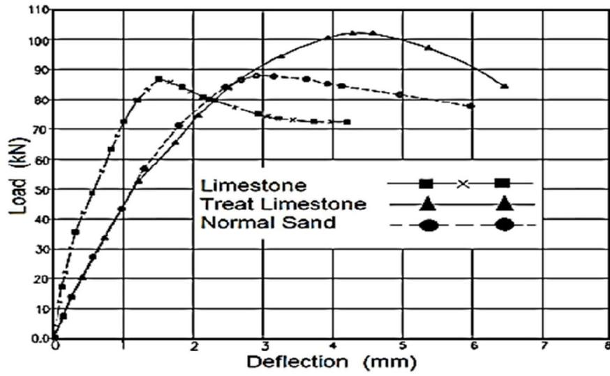
**Figure ( 13 ) :** Curve of load application versus displacement in the test.
