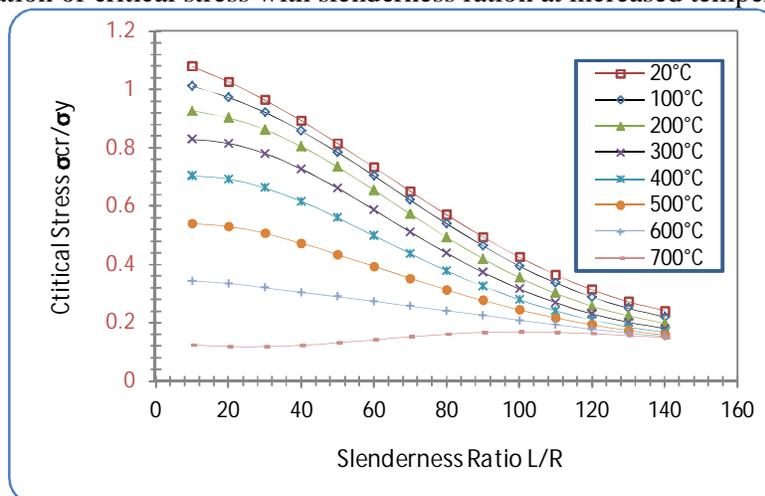
Figure 14: Variation of critical stress with slenderness ration at increased temperature for series 4.
