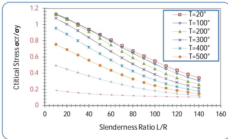
Figure 13: Variation of critical stress with slenderness ration at increased temperature for series 2.
