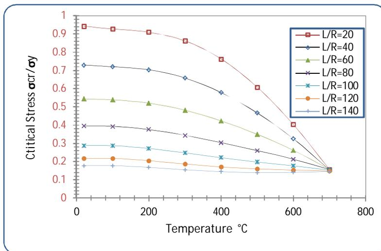
Figure 19: Variation of critical stress with temperature for series 6.
