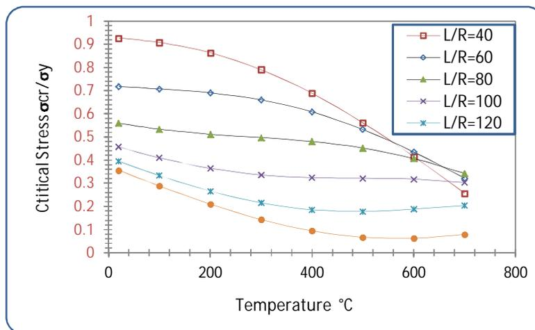
Figure 16: Variation of critical stress with temperature for series 1.
