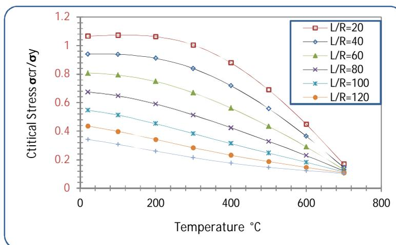
Figure 17: Variation of critical stress with temperature for series 2.
