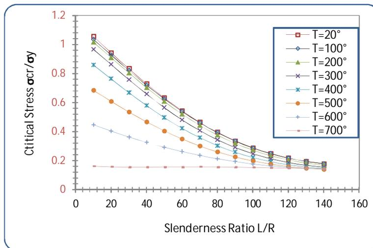
Figure 15: Variation of critical stress with slenderness ration at increased temperature for series 6.
