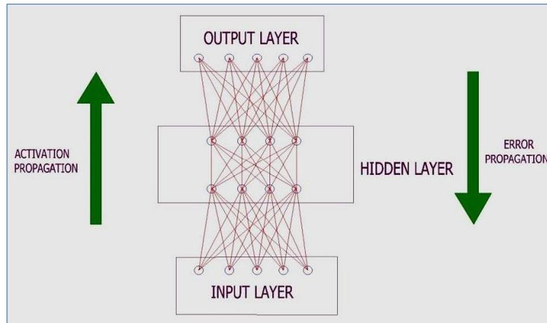
Figure 1: Back-propagation technique of neural network.
