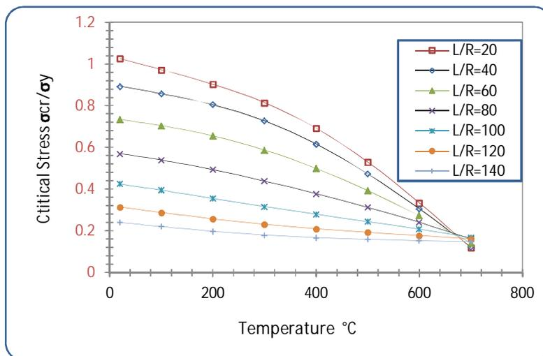
Figure 18: Variation of critical stress with temperature for series 4.
