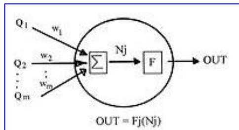
Figure 2: The schematic representation of network processing within an artificial neuron.
