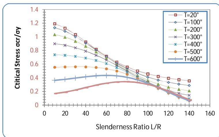
Figure 12: Variation of critical stress with slenderness ratio at increased temperature for series 1.
