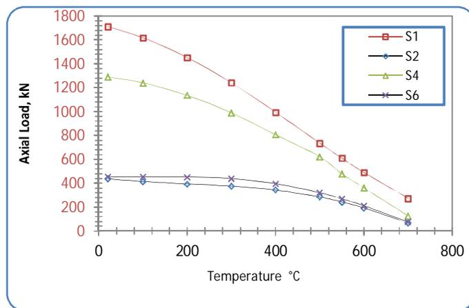
Figure 11: ANN-model results for series (S1, S2, S4, and S6) at different temperature.
