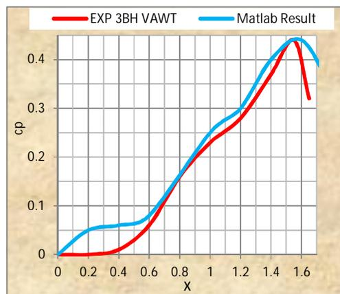
Figure (14) Cp for two blades VAWT Figure (15) Cp for three blades VAWT
