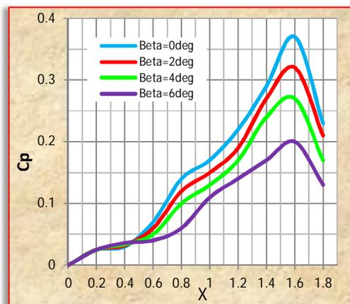
Figure (9) Blade pitch angle (beta) Effect on Cp
