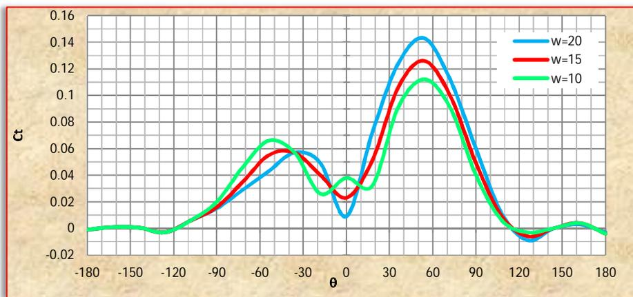
Figure (10) Torque coefficient as a function of blade azimuth angle ( $\theta$ ) for different angular velocity ( $\omega$ )
