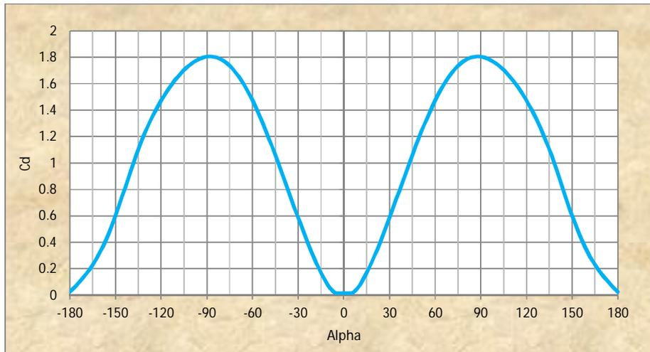
Figure (13) Drag coefficient vs. angle of attack
