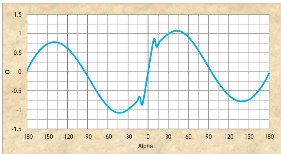
Figure (12) Lift coefficient vs. angle of attack
