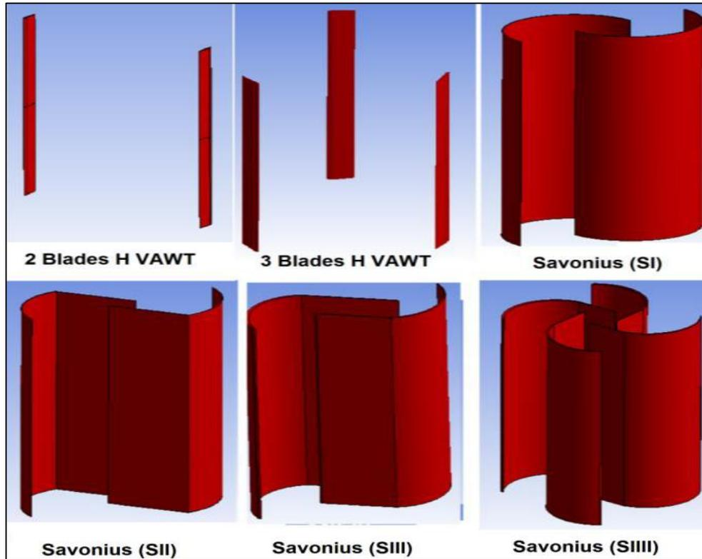
Figure (3) the designed geometries of VAWT rotor
