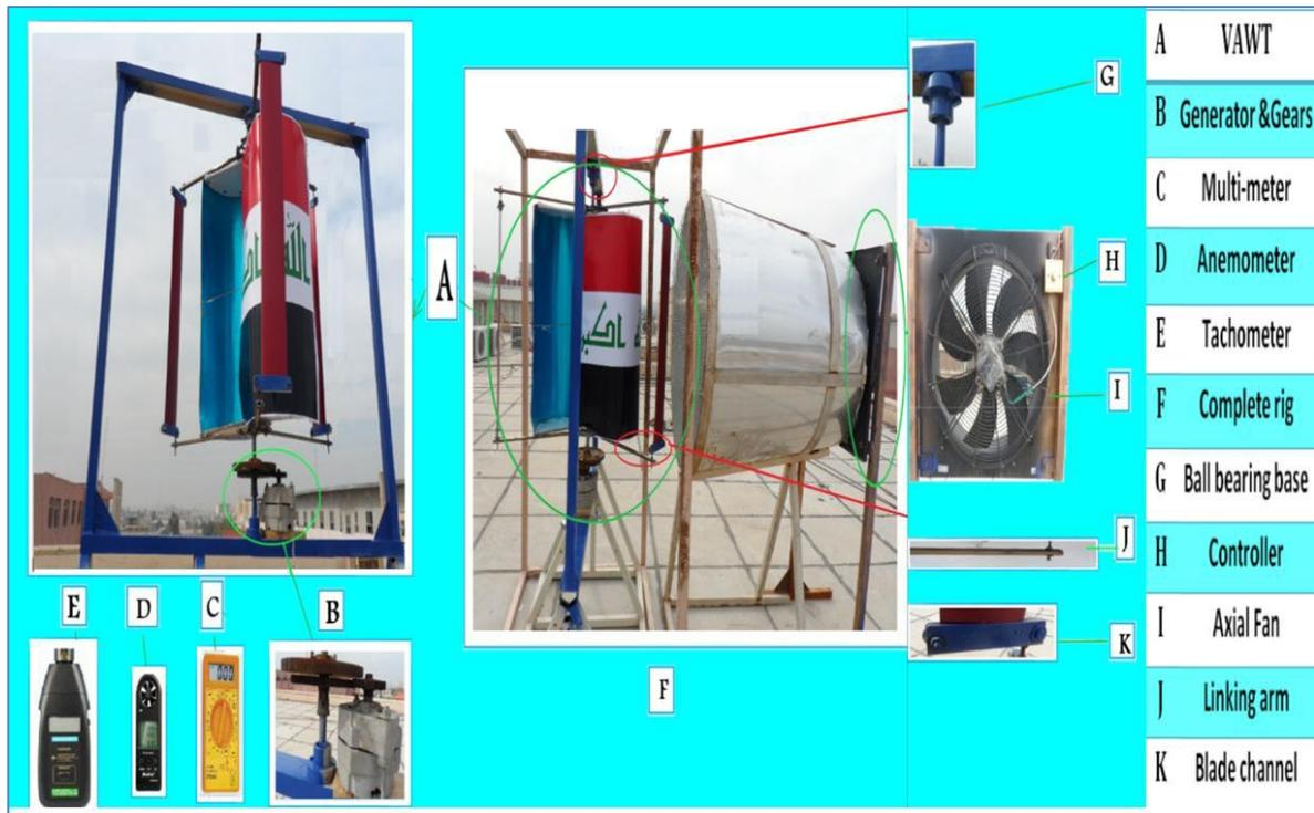
Figure (1): The designed small vertical axis wind turbine
