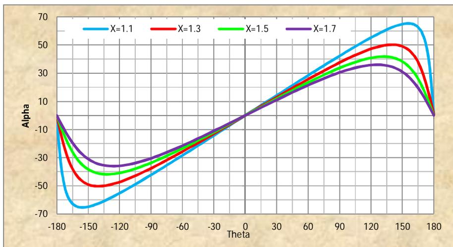
Figure (11) Effect of tip speed ratio on alpha
