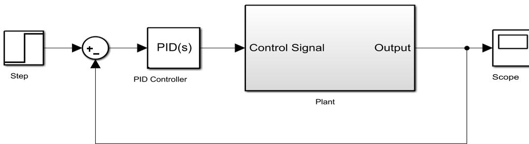
Figure 4. Block diagram of feedback control system with a PID controller simulated by Matlab-Simulink
