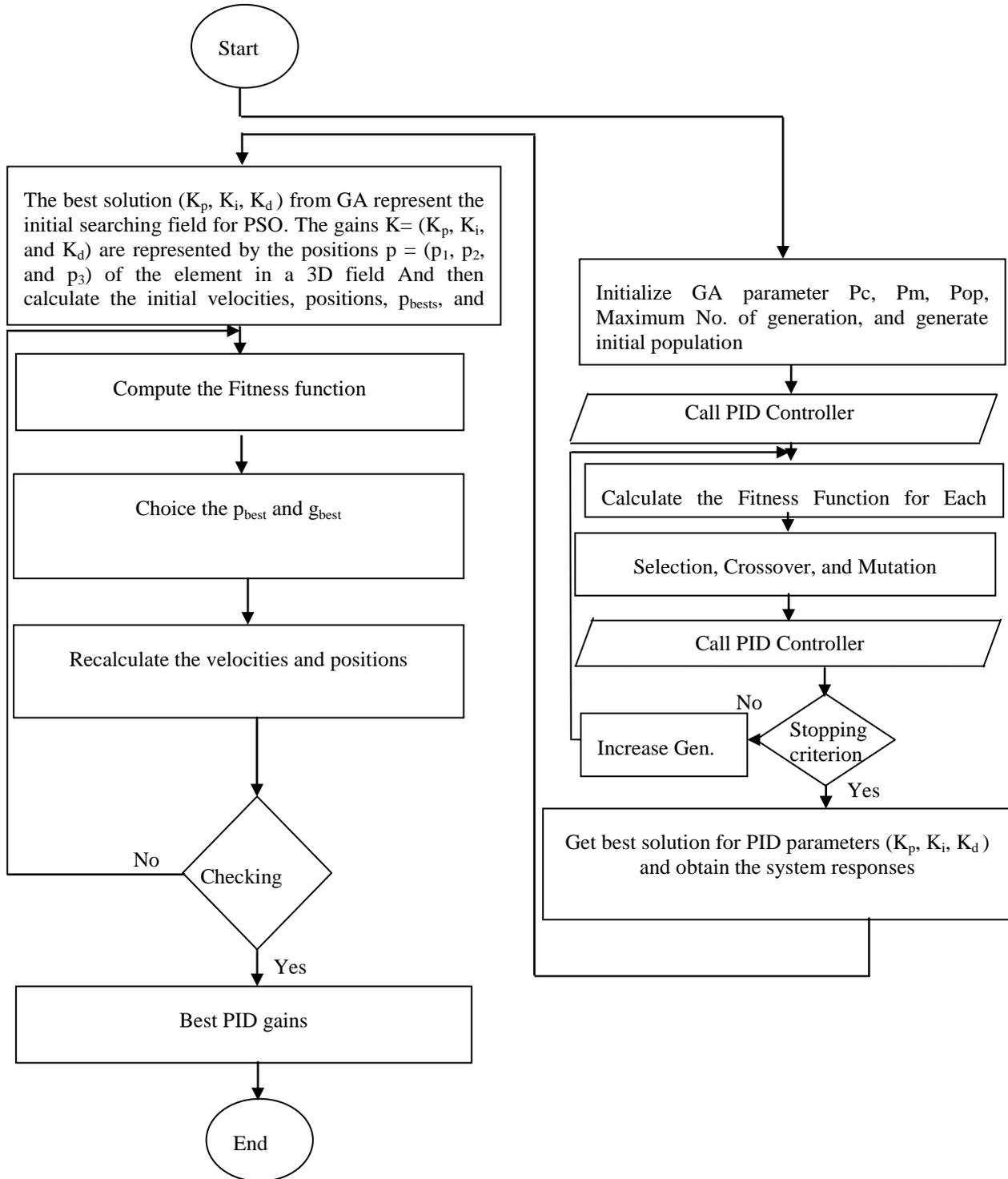
Figure 3. Flowchart of the proposed controller PSO-FGA-PID
