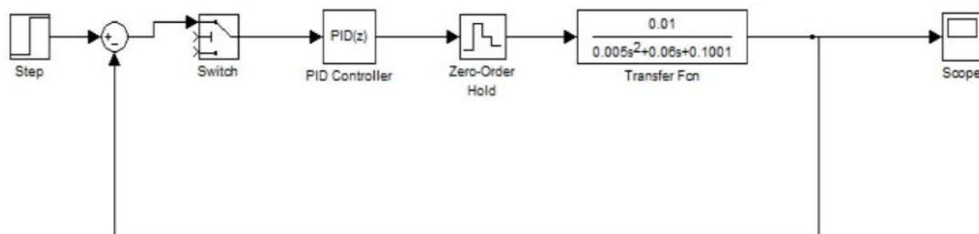
Figure 10. Feedback DC motor control system simulated in Matlab simulank
