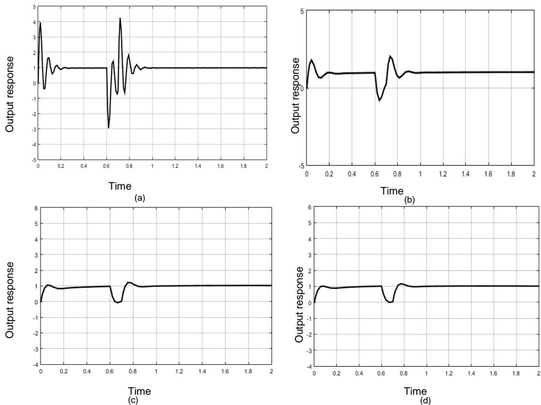
Figure 8. The responses of LTI system with sudan change (a) without controller (b) with PID controller (c) with FGA-PID (d) with PSO-FGA-PID
