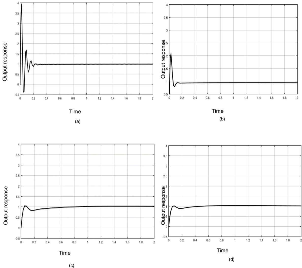
Figure 6 . The responses of LTI system (a) without controller (b) with PID controller (c) with FGA-PID (d) with PSO-FGA-PID
