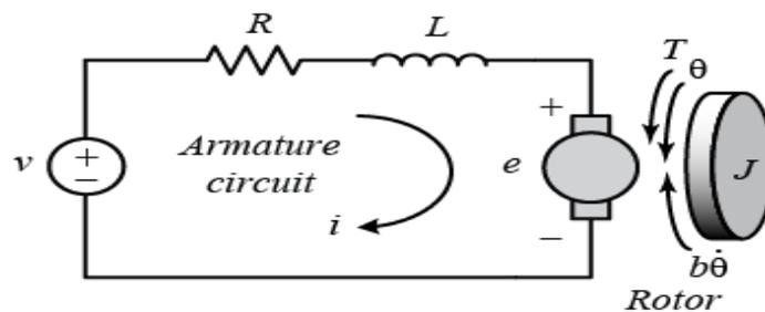
Figure 9. The Schematic of the DC Motor
