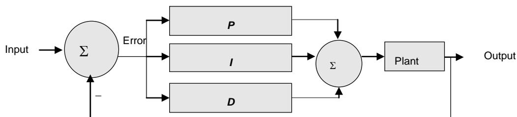
Figure 1. The system with a PID
