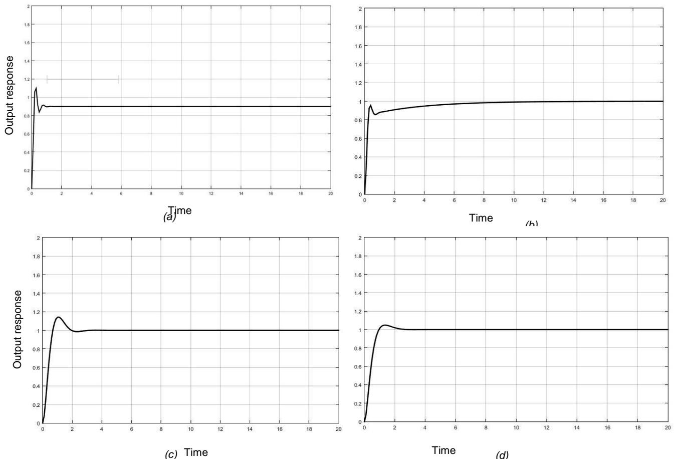
Figure 11 . The responses of DC motor system (a) without controller (b) with PID controller (c) with FGA-PID (d) with PSO-FGA-PID
