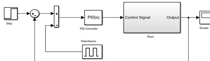
Figure 7. Simulation of system subjected to a disturbance
