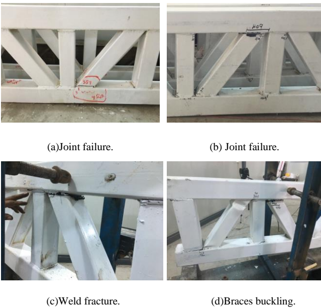
Figure 7: Modes of failure.
