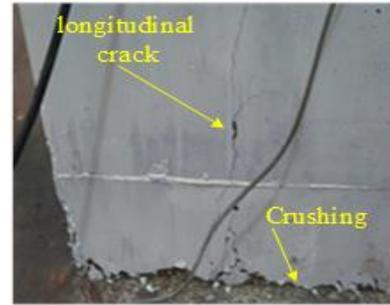
Figure 7 The failure mode of specimens.
