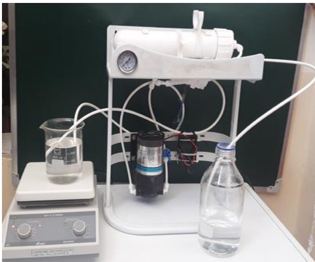
Figure 2. Reverse Osmosis Unit
