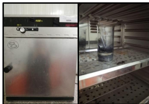
Figure 1. Photographic picture of the apparatus used for coating sand with graphene oxide.
