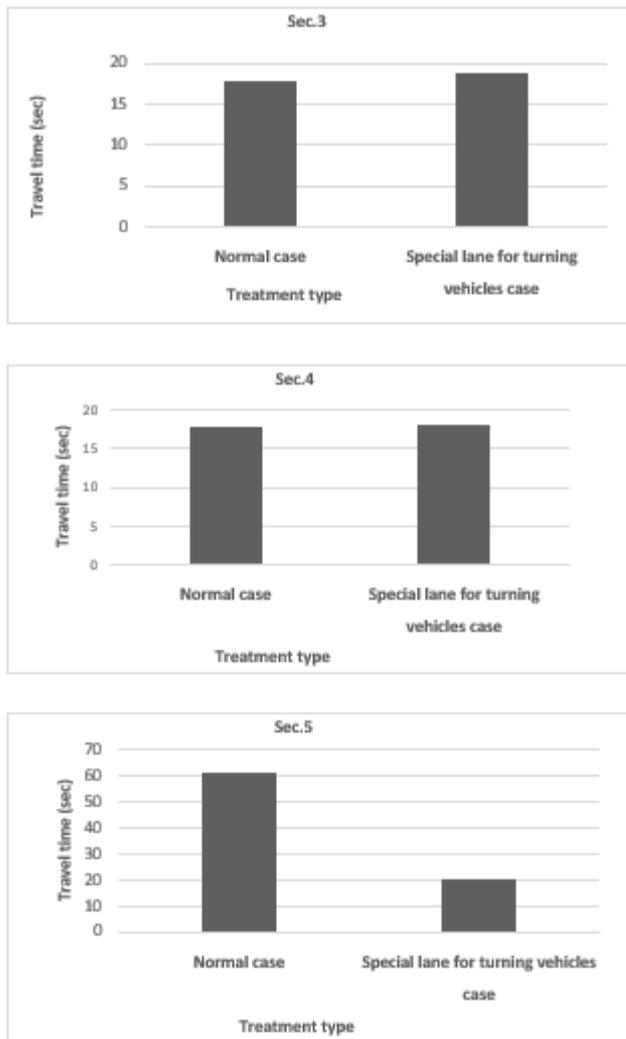
**Figure 8.** The effect of using special lane for turning vehicle on the travel time.
