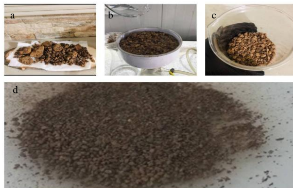
Figure 3. Photographic picture of the steps of preparation of the polymer. a. The polymer was broken into a large spatula, b. The polymer was rinsed in DI water many times; c. A mechanical mill was used to grind the polymer into particles ranging in size from 0.5 to 3 mm; d. The produced polymer was dried in the sieve by putting the material in a drying oven at 42°C.
