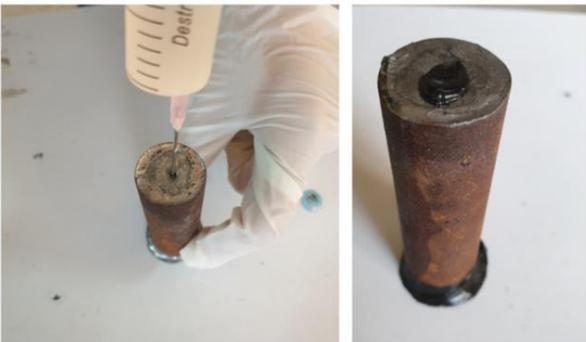
Figure 3. Injecting melting paraffin wax in capsule.
