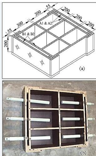
**Figure 1.** Pull-out test: a) Mould fabrication, b) Preparing for casting
