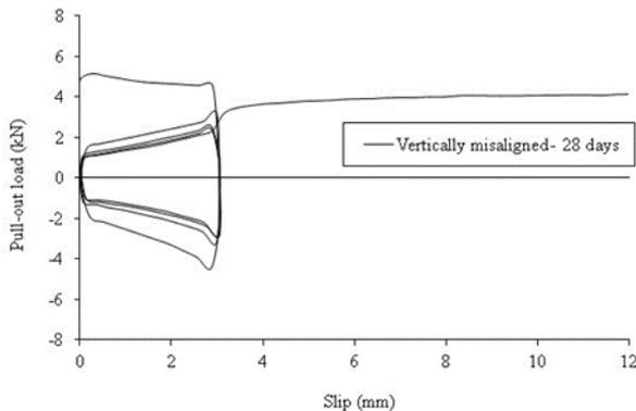
Figure 4. Cyclic pull-out load vs. slip distance for vertically misaligned dowel bar
