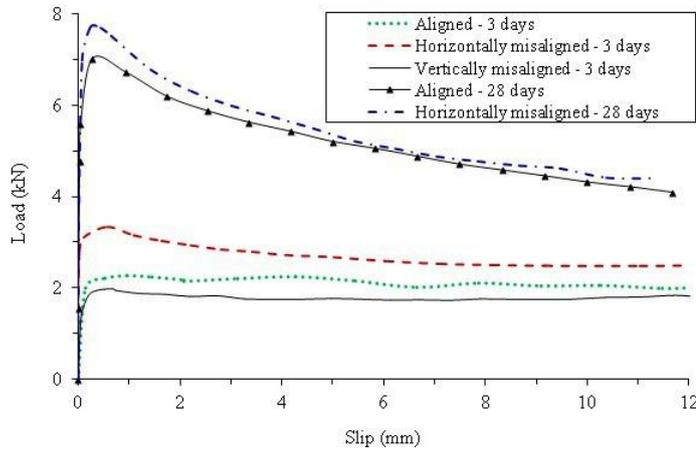
Figure 3. Pull-out load vs. slip distance at ages of 3 and 28 days
