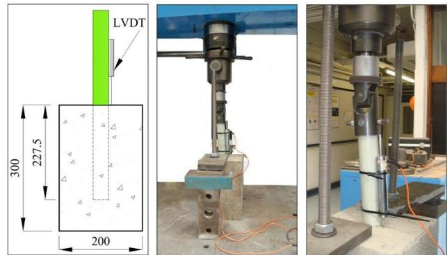
**Figure 2.** Pull-out test, specimen dimensions, and test setup
