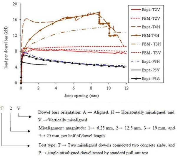
Figure 5. Comparison of pull-out load per dowel for specimens containing two concrete slabs connection ting by two misaligned GFRP dowel bars across the joint with pull-out from standard pull-out test at age of 28 days. Note: the nomenclatures in the legend were adopted in the figure above.
