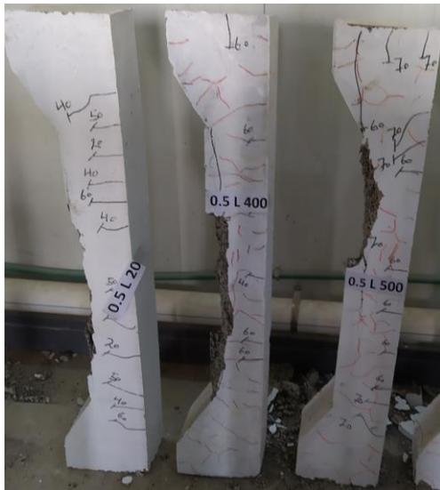
Figure 9. Column specimen failure for 0.5L20, 0.5L400, 0.5L500
