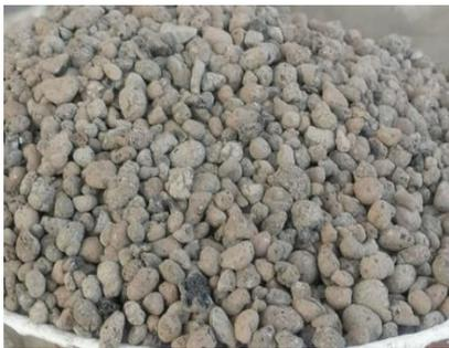
**Figure 1.** Lightweight expanded clay aggregate (LECA) was used in the current study.
