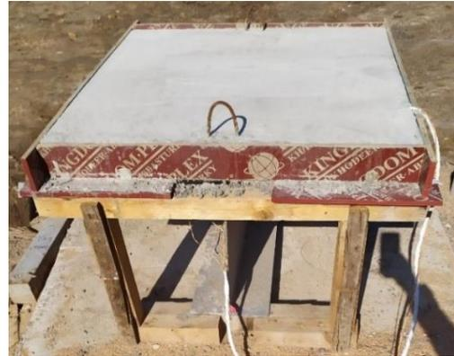
**Figure 2.** Specimen after casting.
