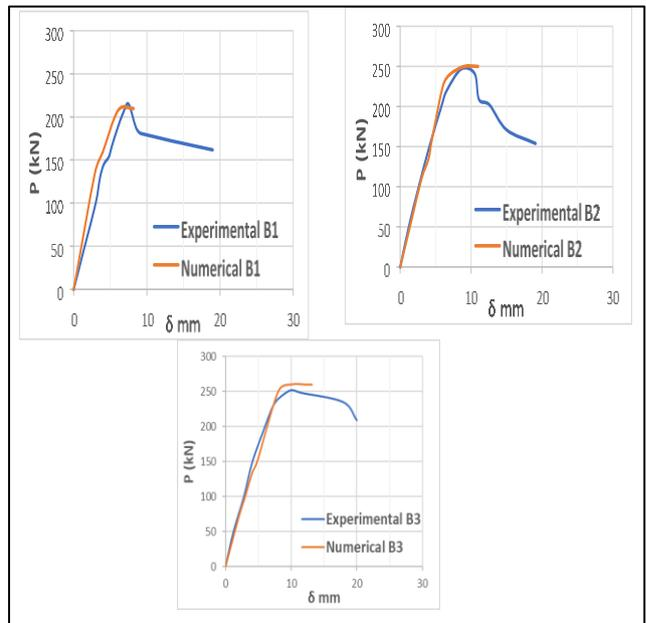
Figure 4. The load-deflection of the beam with different pattern stirrups
