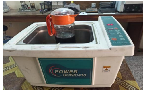
Figure 3. An ultrasonic bath (Model power sonic 410) was used for nanofluid preparation.
