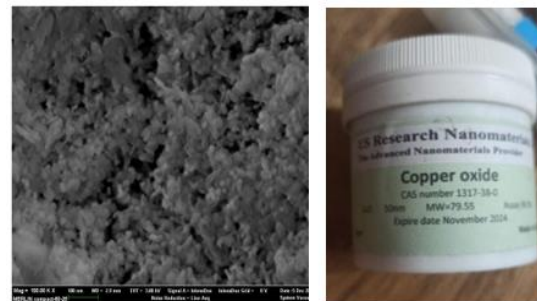
Figure 4. SEM image of 25 nm dry OF CuO nanopowder.
