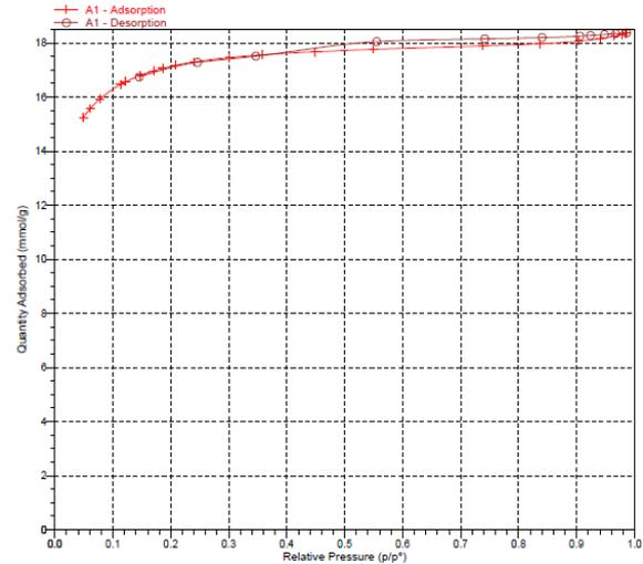
**Figure 3. N2 adsorption-desorption isotherm of AC Results of experimental design**
