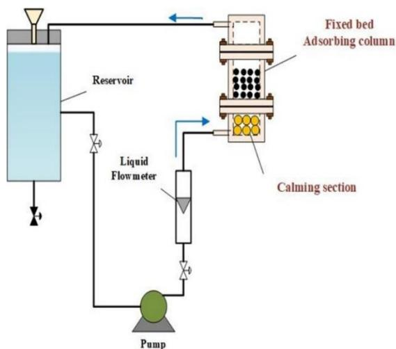
**Figure 1. Schematic diagram of the chemical system by adsorption process.**
