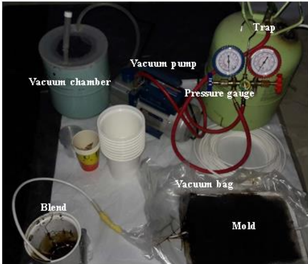
Figure 2. Vacuum infusion technique
