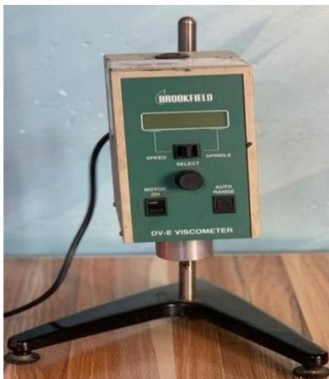
Figure 1. DV-E Viscometer used for viscosity measurements.
