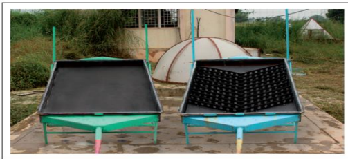
Figure 2. Flat-platelet solar air collector and baffles V-shape tailored plate. [4]
