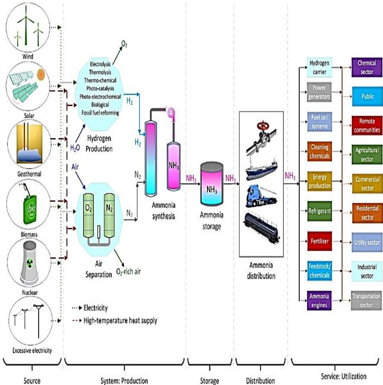
Figure 3. Ammonia life cycle from production to utilization [7]
