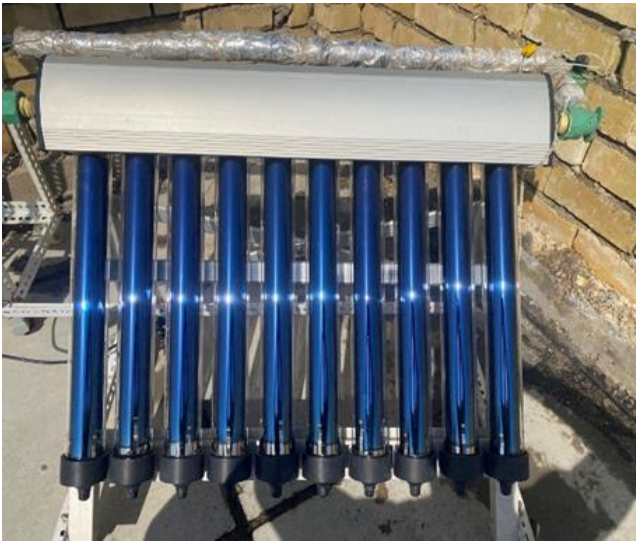
Figure 1. A photograph showing the ten evacuated tubes used in the solar collector
