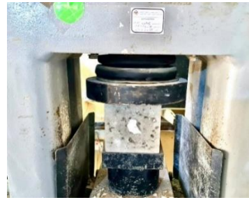
Figure 4. The compressive strength test
