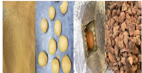
Figure 2. The preparation steps of the montmorillonite coarse aggregate
