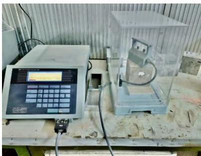
Figure 3. The thermal conductivity test
