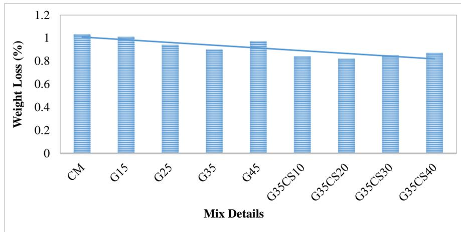
Figure 3. Sulphate attack test results
