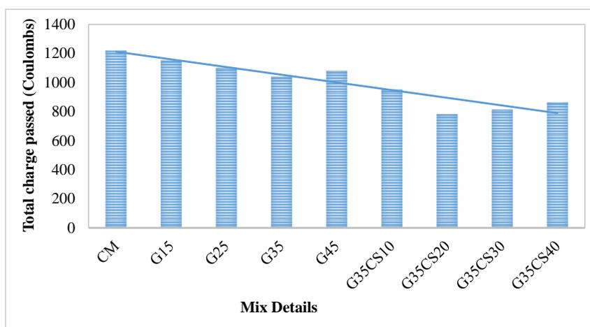
**Figure 1.** RCPT Test results of different mixes.
