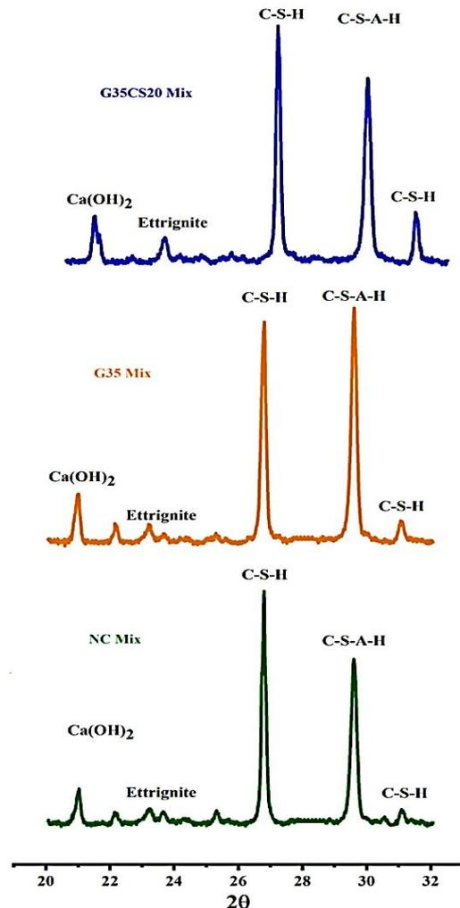
Figure 5. XRD Analysis of different mixes
