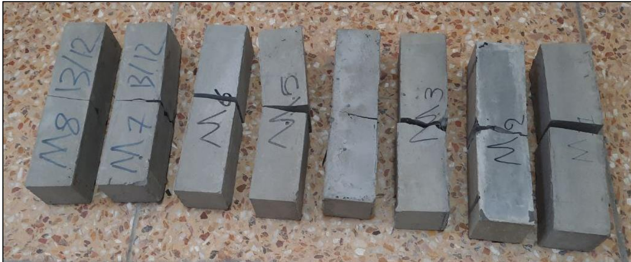
Figure 14. The broken prism specimens after the test
