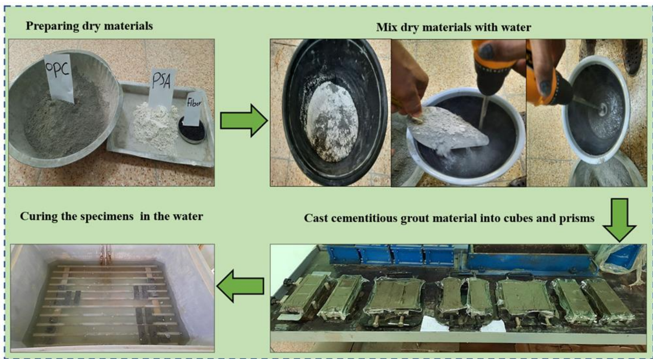
Figure 8. The cementitious grout preparation
