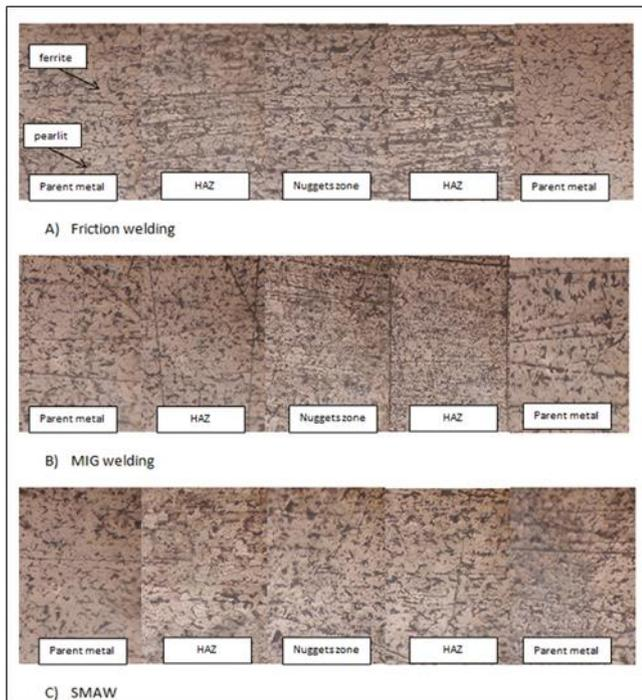
**Figure7.** Microstructure along the welded rods at different welding zones (X164) for (a) friction weldments; (b) MIG weldments; and (c) SMAW
