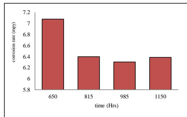
**Figure 9.** Corrosion rates for SMAW weldments
