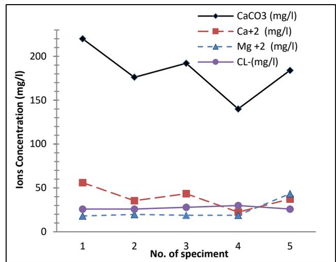
Figure 5. CaCO<sub>3</sub>, Ca<sup>+2</sup>, Mg<sup>+2</sup>, and Cl<sup>-</sup> ions concentrations for the tap water (1) and the corrosive solutions after 1150 hours of the immersion of weldments: (2) friction weldments. (3) SMAW weldments. (4) MIG weldments, and (5) base metal samples.
