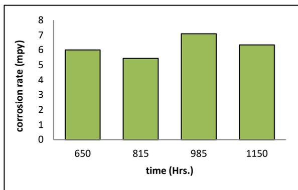
Figure 10. Corrosion rates for MIG weldments
