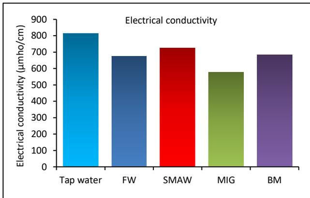
Figure 4. Electrical conductivity for the tap water (1) and the corrosive solutions after 1150 hours of the immersion of weldments:
