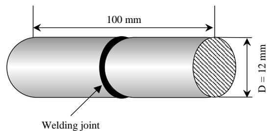
**Figure 1.** Welded sample dimensions before the immersion test
