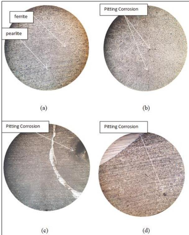
**Figure 6.** Microstructure of the parent metal and the different weldments at the nugget zone ( X100 ). (a) parent metal; (b) friction weldments; (c) SMAW weldments; and (d) MIG weldments
