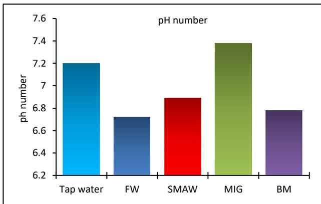
Figure 3. pH numbers for the tap water and the corrosive solutions after 1150 hours of the immersion of weldments
