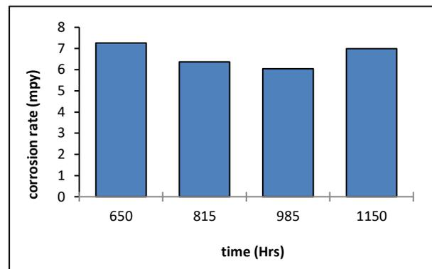
**Figure 8.** Corrosion rates for friction weldments
