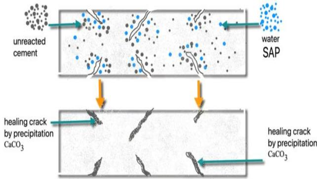
Figure 3. The mechanism of SAP within the concrete
