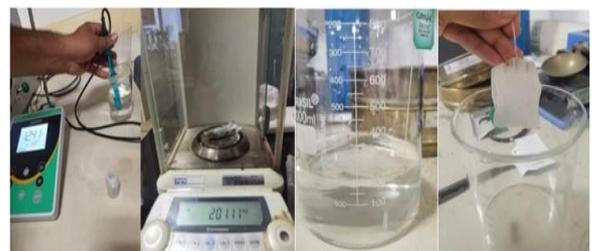
**Figure 2.** Method of conducting the water absorption by the SAP
