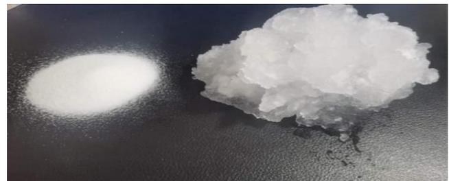
**Figure 1.** Superabsorbent polymer (SAP) in a dry and wet state
