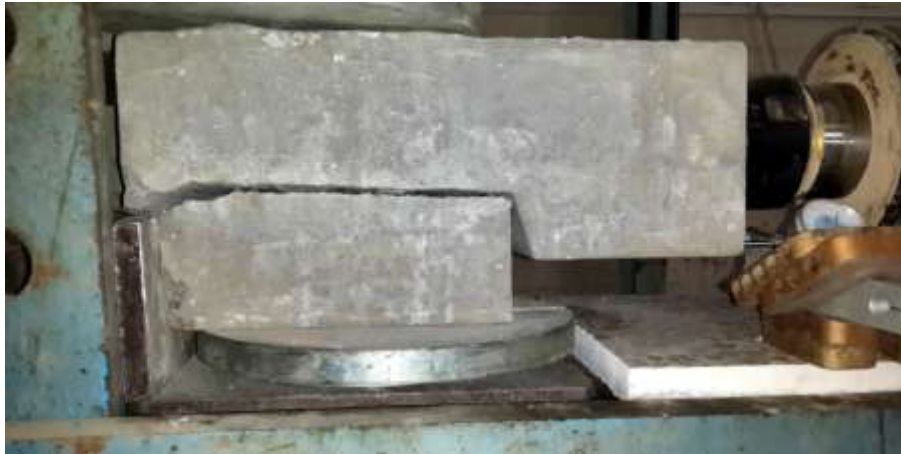
Photo (1): Concrete to concrete shear test
