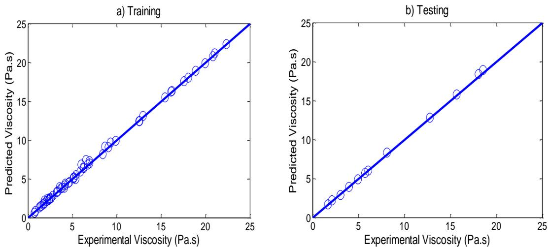
**Figure (10):** The graphical output of the experimental viscosity plotted versus neural network predicted viscosity.
