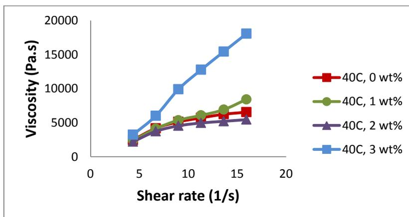
Figure (4): Viscosity of epoxy resin modified by pomegranate peel for different concentration vs. shear rate at 40 °C.
