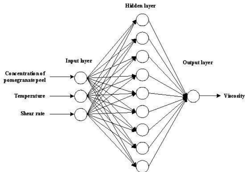
**Figure (1):** The system architecture used in the ANNs models.
