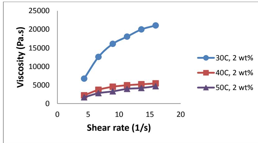
**Figure (8):** Viscosity of epoxy resin modified by pomegranate peel (2 wt%) versus shear rate at different temperatures.
