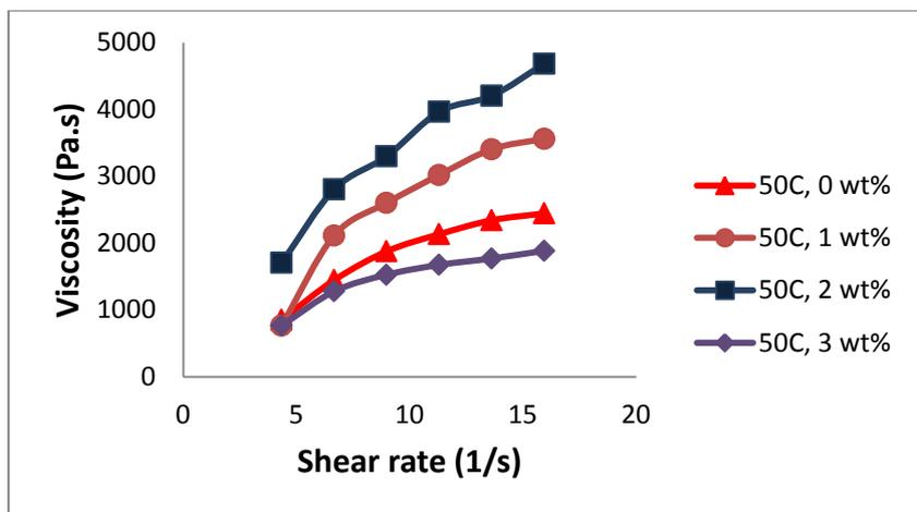
**Figure (5):** Viscosity of epoxy resin modified by pomegranate peel for different concentration vs. shear rate at 50 °C.
