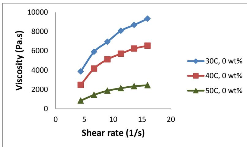
**Figure (6):** Viscosity of epoxy resin modified by pomegranate peel (0 wt%) versus shear rate at different temperatures.
