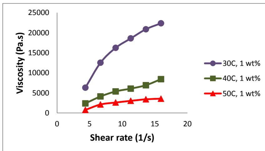
**Figure (7):** Viscosity of epoxy resin modified by pomegranate peel (1 wt%) versus shear rate at different temperatures.
