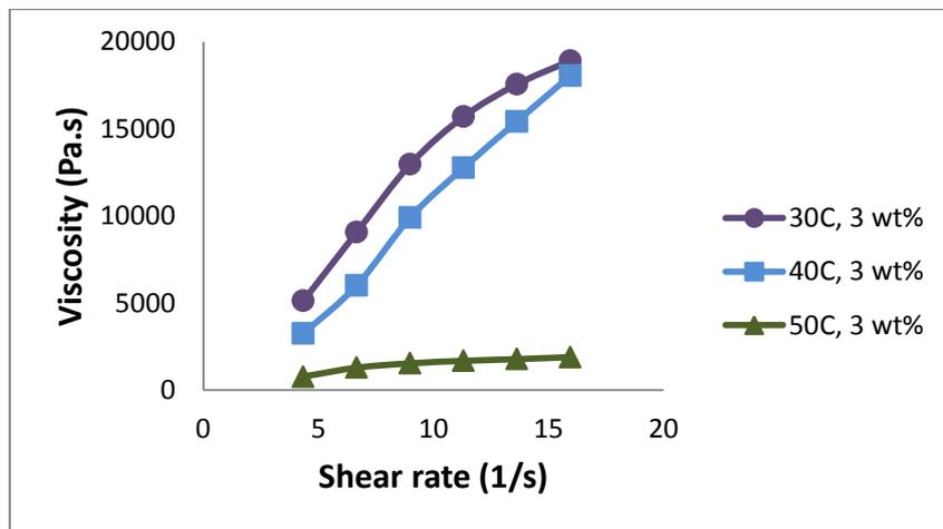
**Figure (9):** Viscosity of epoxy resin modified by pomegranate peel (3 wt%) versus shear rate at different temperatures.
