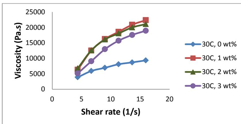
Figure (3): Viscosity of epoxy resin modified by pomegranate peel for different concentration vs. shear rate at 30 °C.
