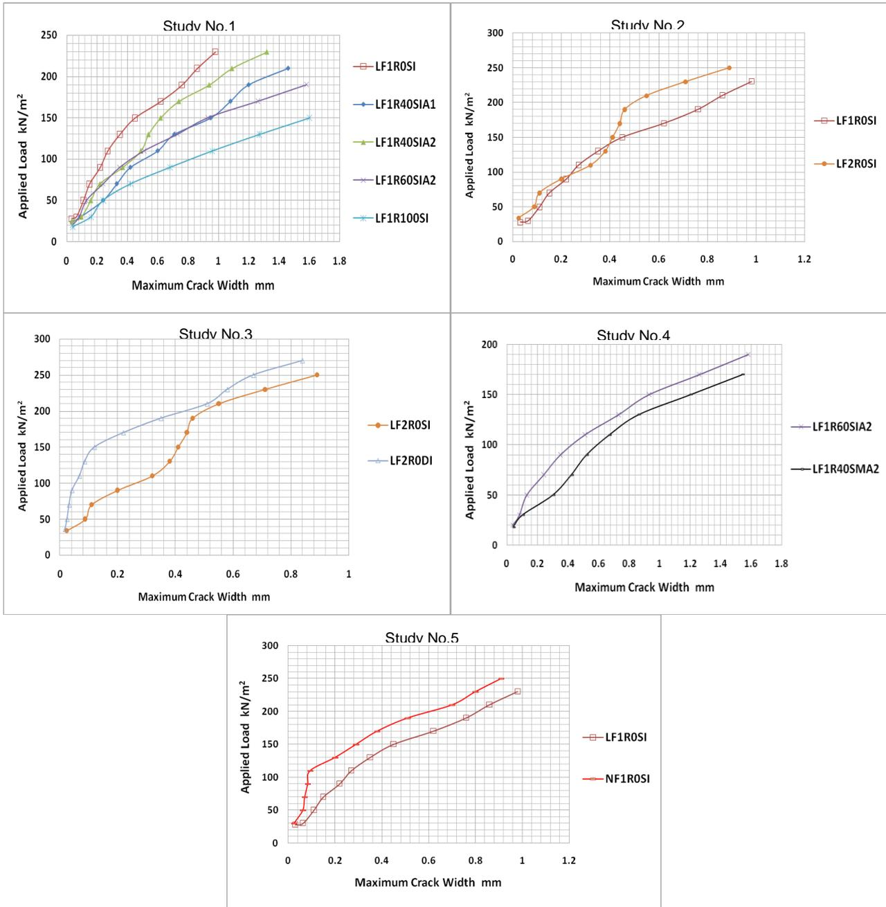
**Figure 4** Maximum crack width versus load for all slab models
