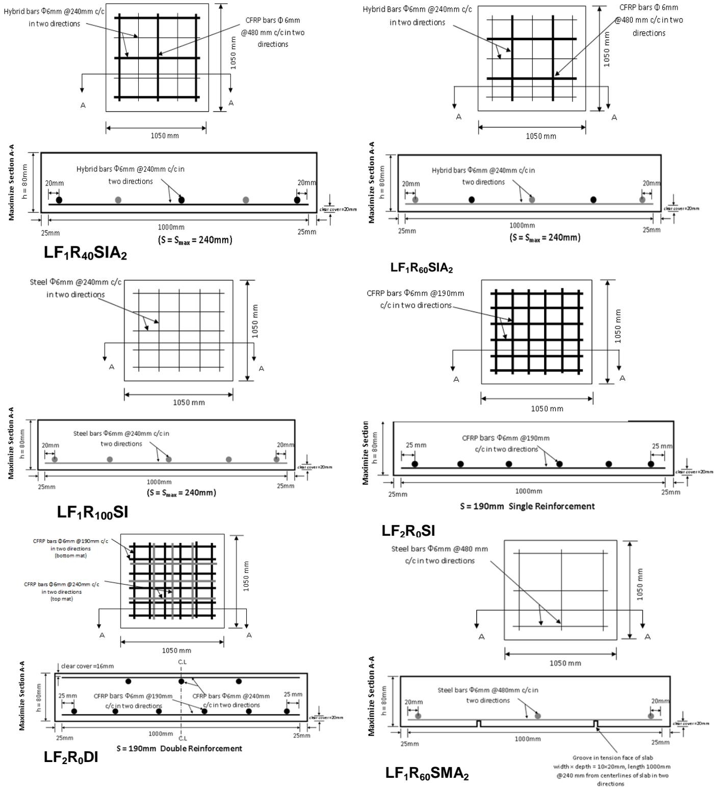
Continued of Figure 2 Details of reinforcement of slab models
