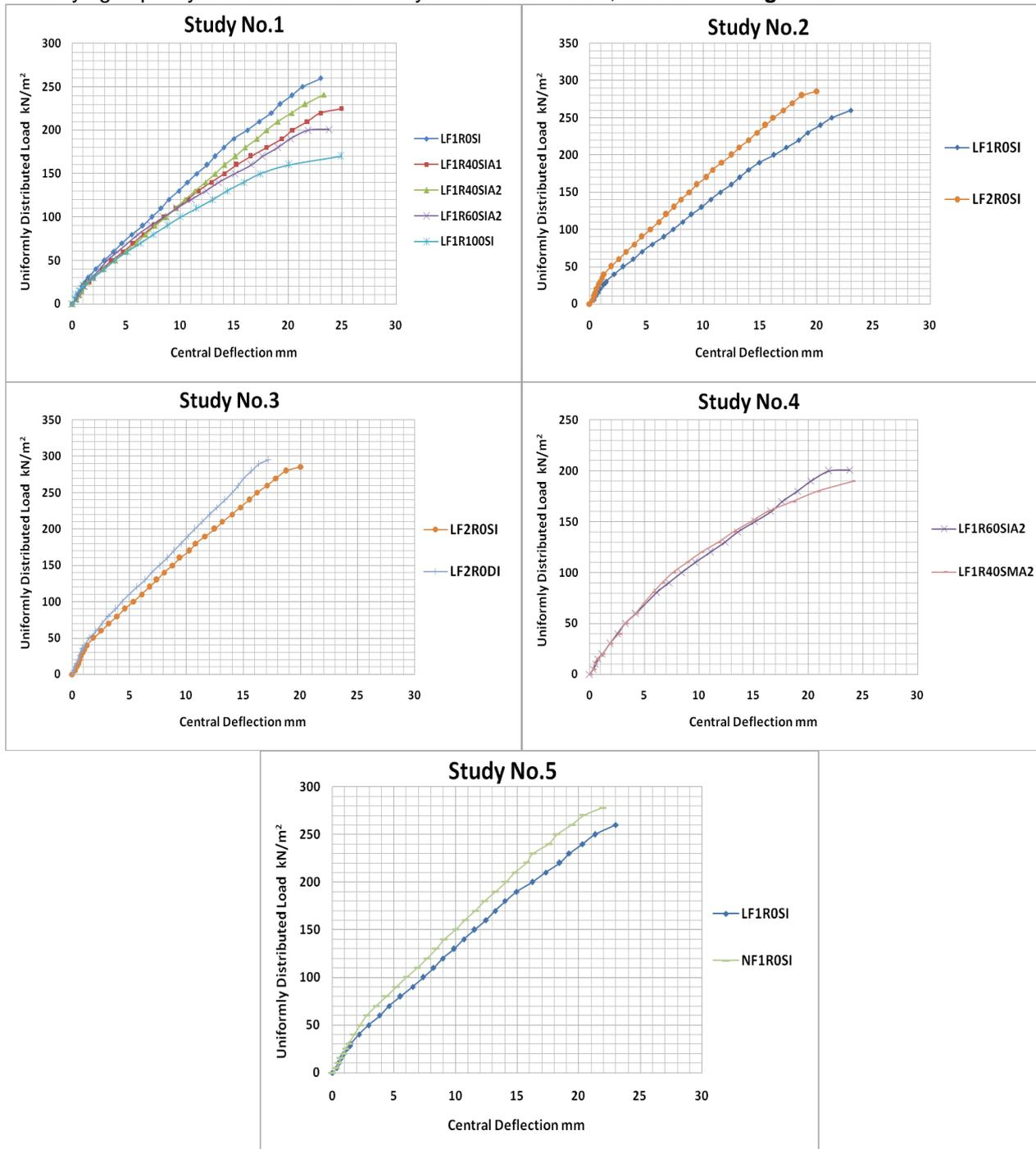
**Figure 5** Load–central deflection curve for all slab models
