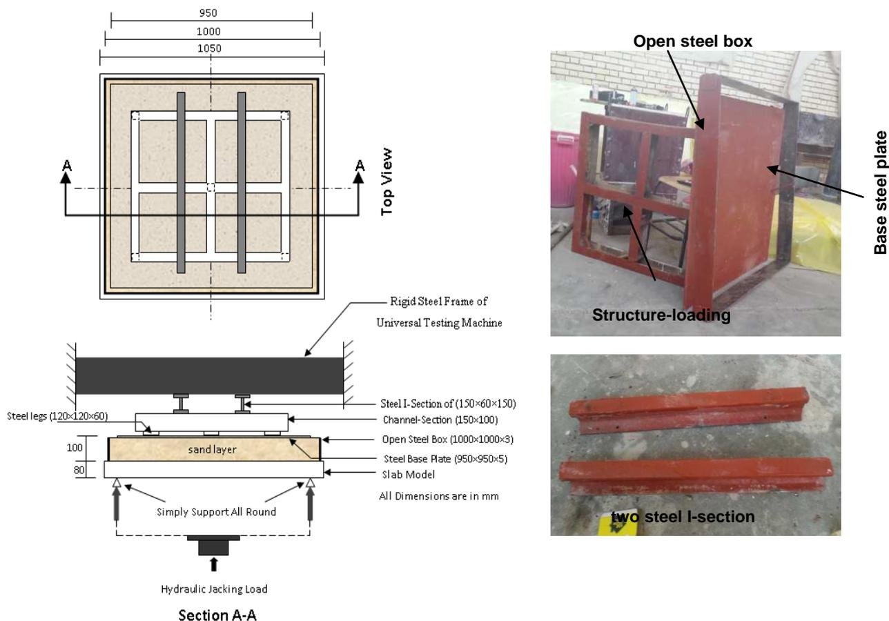
**Figure 3:** Loading system for test slab models under uniformly load.
