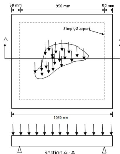
**Figure 1:** Details of dimensions concrete slab models.
