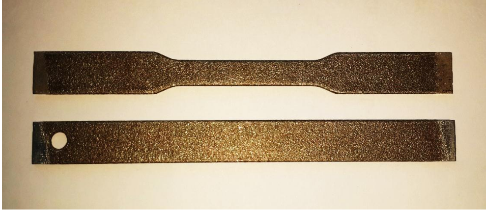
Figure 3: tensile test specimen and fatigue test specimen after shot peened process.
