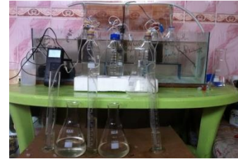
Figure 4. Lap scale anaerobic digesters.
