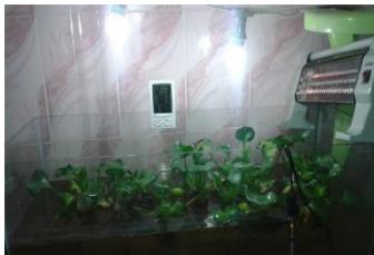
Figure 2. The treatment of wastewater via water hyacinth.
