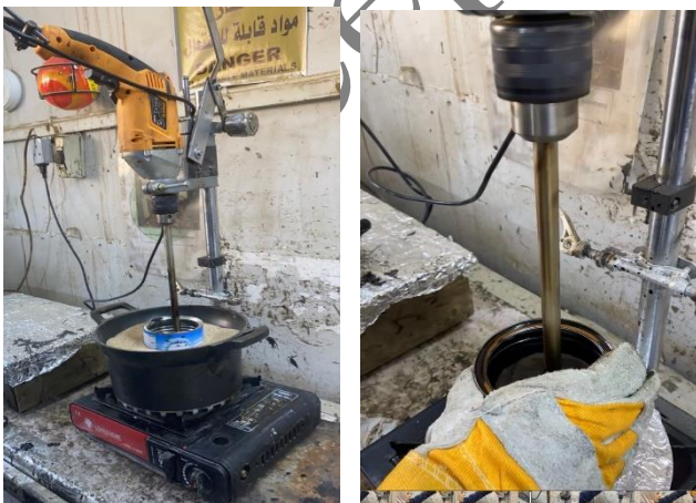
Figure 2. Tire crumb rubber modified preparation
