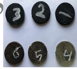
Fig. 7. The hardness test specimen (d:12, h:24) mm.
