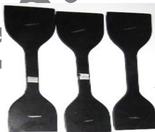
Fig. 12. Dumbbell shape specimen. 2 mm thickness and 165 mm effective length.
