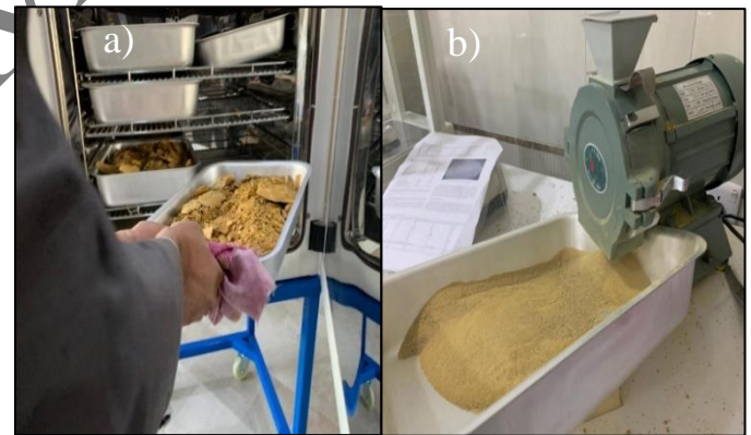
Figure 1. The preparation process of bentonite, a) the Drying process, and b) the Grinding process.
